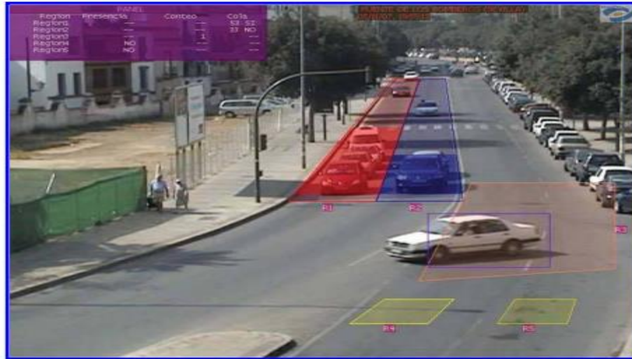
Figure. Detection areas in the installed prototype: details of the queue and the directional regions behavior
