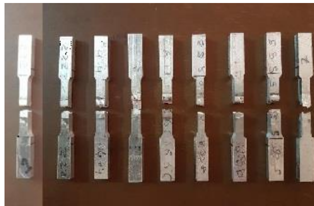
Figure 10. Tensile specimens AA 7075 after tensile testing (1)
