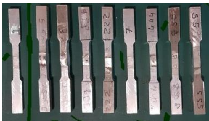
Figure 8. Prepared tensile specimen of AA 7075 as per ASTM E8 Standard (1)
