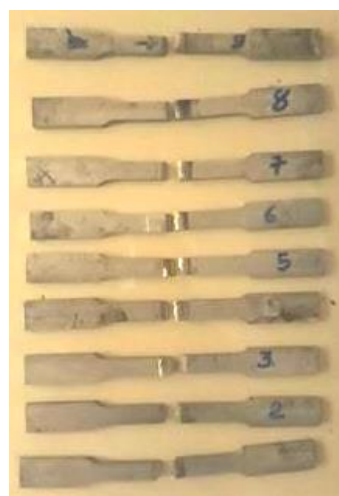
Figure 11. Tensile specimens AA 6061 after tensile testing (2)
